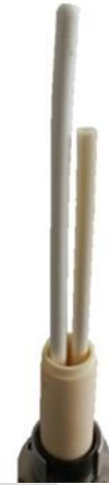
Fig. 4 An oxygen filter (left, slightly deformed after a test series) as mounted in the set-up. The protective tube was removed but for the lowest segment. To the right of the filter is an inlet tube for the feed gas.
