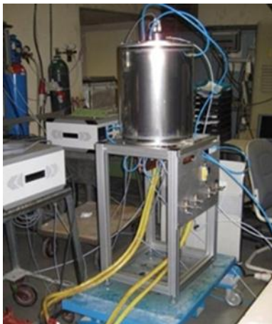
Fig. 1 The oxygen filter test bench. The components are contained in a steel vessel.
