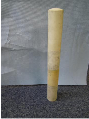
Fig. 3 A protective tube with four segments after use in the test bench.
