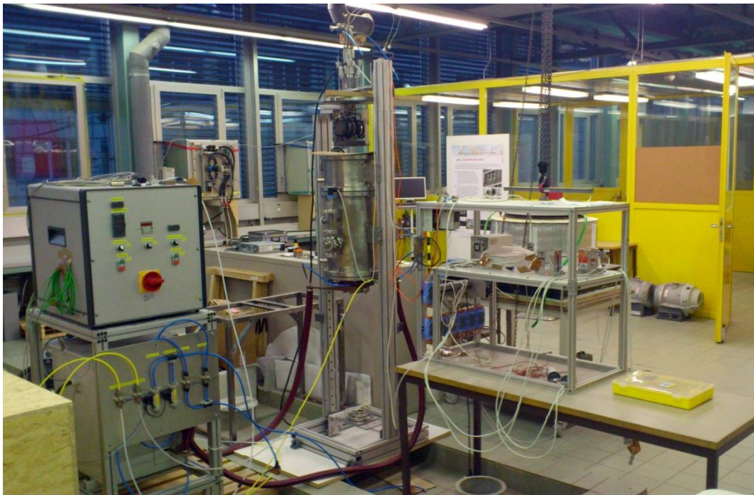
Figure 5 The furnace for proof of concept installed at HEPIA 10 in the laboratory of H2 Power Technical Center in 2014. At HEPIA, compared to IKTS, much more lab space was available for the installation. The hydrogen generator is mounted in the alu-profile rack in the middle of the picture.
