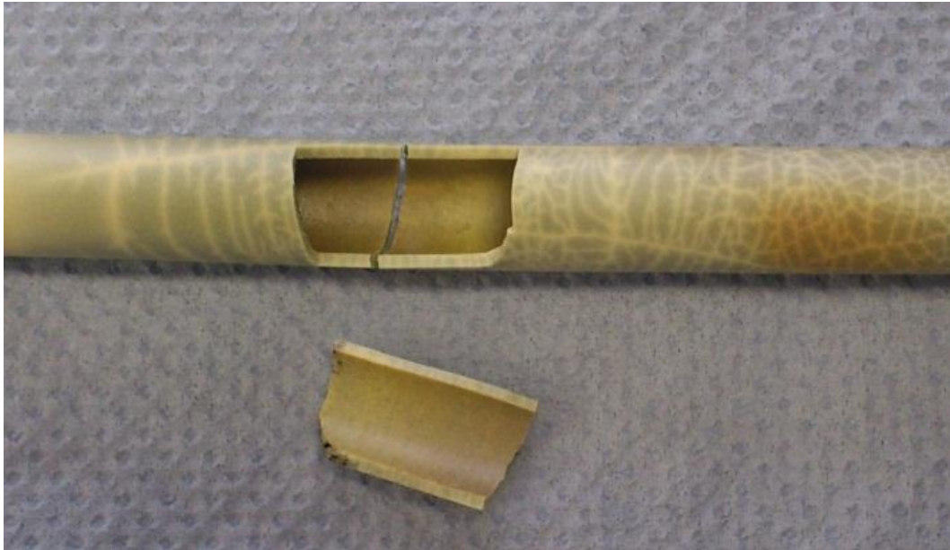
Figure 4 Stress pattern and cracking observed in a region with a high thermal gradient but a comparatively low absolute temperature.
